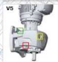
6 interchangeable plugs, including one breather plug and a level plug. Level and breather plug must be positioned according to this chart
